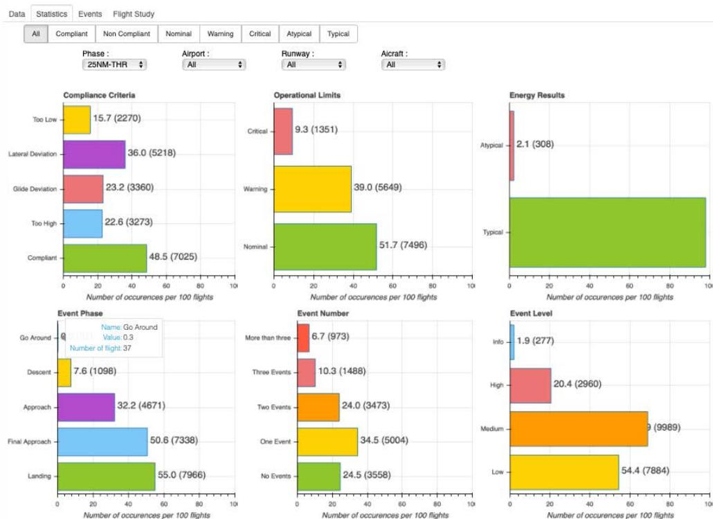
**Fig. E.2** Statistics section of TAPAS prototype software. It provides information on operational statistics such as the compliance or the average number of monitoring events per 100 flights.
