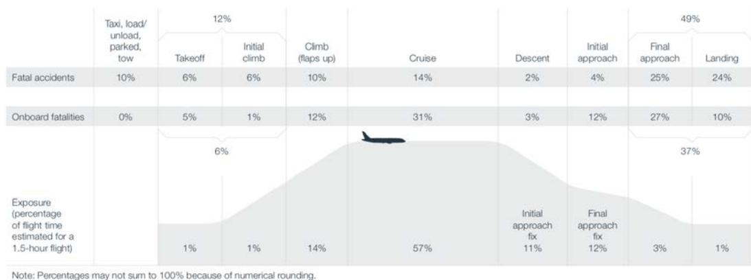
**Fig. 1.2** Accident rates and on-board fatalities per flight phases [1]
