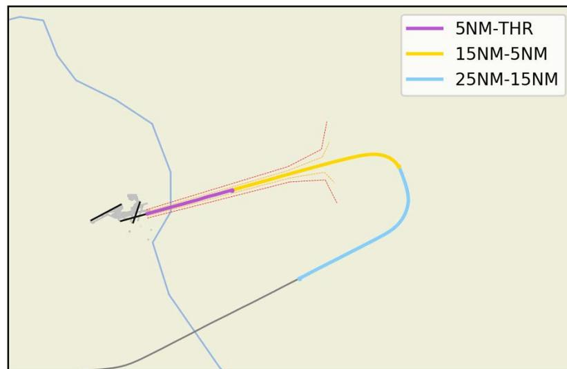
**Fig. 3.5** The three phases on a flight landing at Paris Orly Airport.
