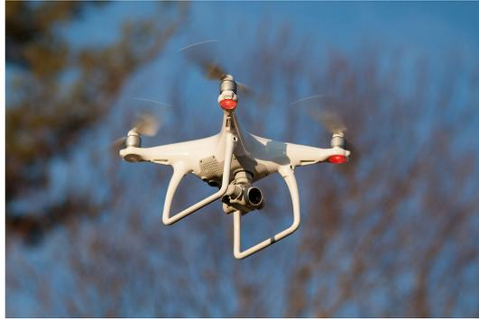
Figure 2.1: DJI Phantom 4 quadcopter
