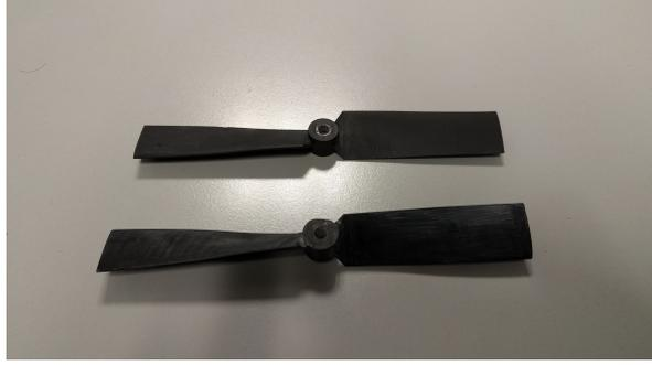
Figure 3.6: 3D Printed NACA propellers
