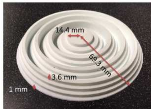
Figure 3.20: 3-D printed Fresnel lens [122].
