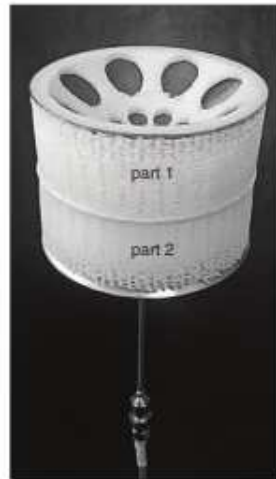
Figure 3.15: Biconical antenna with dielectric lens.
