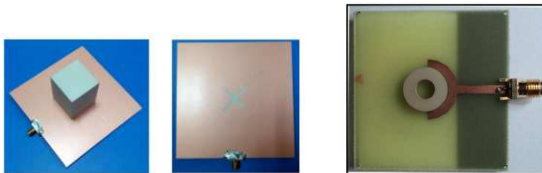
(a) Cross-slot-coupled dual-band circularly polarized DRA [50].
