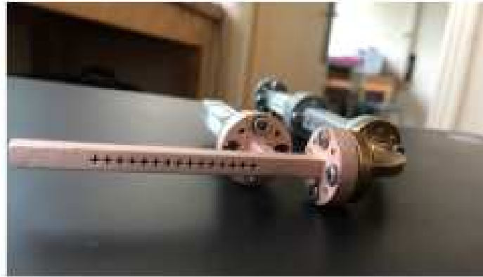
(a) Dual-polarized leaky-wave antenna [114].
