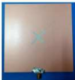
(a) Cross-slot-coupled dual-band circularly polarized DRA [50].
