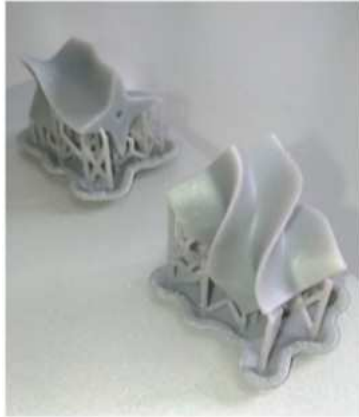
Figure 3.24: Super-shaped DRAs for 5G applications using Stereolithography [129].
