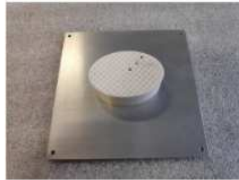
(b) Elliptical DRA in circular polarization [77].
