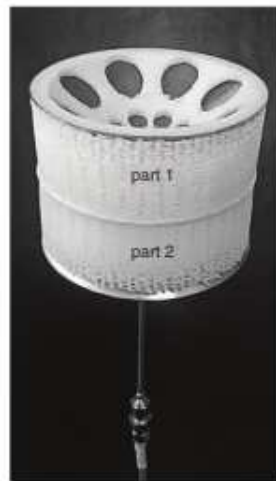
Figure 3.15: Biconical antenna with dielectric lens.
