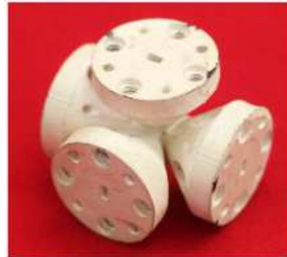
(b) Metallized millimeter-wave waveguide [103].
