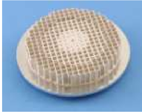
Figure 3.22: 3-D-printed wideband multi-ring DRA [128].
