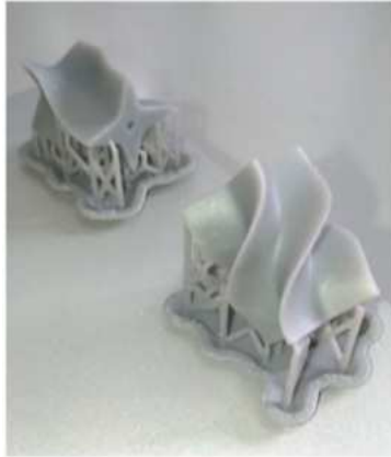
Figure 3.24: Super-shaped DRAs for 5G applications using Stereolithography [129].
