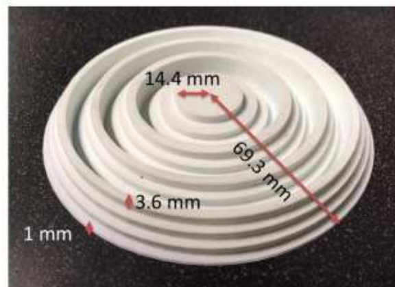
Figure 3.20: 3-D printed Fresnel lens [122].
