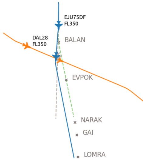
Figure 2. The blue trajectory is deviated. Predictions are represented with dashed lines, the straight-line prediction in grey and the one following the flight plan in green.
