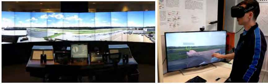
Fig. 2. Typical Remote Tower room (left). The immersive environment for the Remote Tower concept (right).
