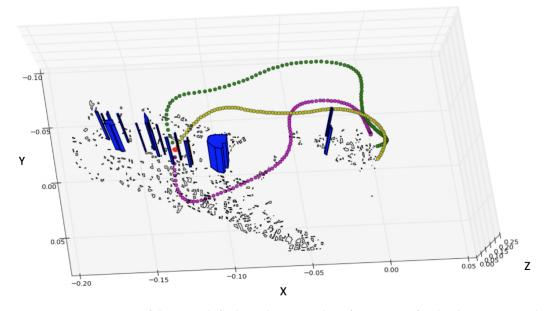
**Figure 9.** Computation of the smooth flight paths. Input: list of waypoints for the three computed flight paths present in Figure 8. Output: list of waypoints for the three computed smooth flight paths.
