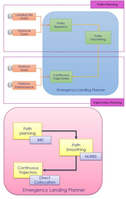
Figure 11. Emergency landing planner architecture.
