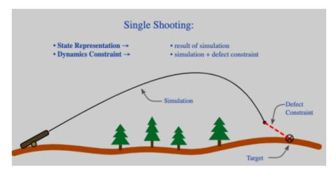
**Figure 4.** Single shooting scheme [39]. It approximates the trajectory using a single simulation: fire the cannon, check where the ball landed, adjust the initial speed, and repeat.
