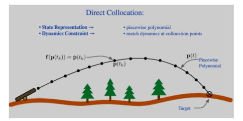
**Figure 6.** Collocation shooting scheme [39]. The trajectory is approximated using a piecewise polynomial. Physics is satisfied by requiring that the dynamics match the derivative of the polynomial at each collocation point.
