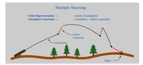
**Figure 5.** Multiple shooting sheme [39]. It works by breaking the problem into smaller ones and solving them parallelly. In the end, each segment is constrained to connect to the previous one.
