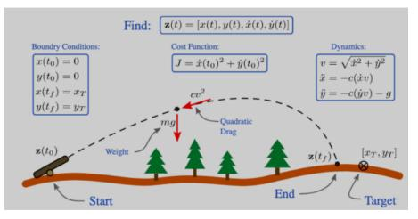
**Figure 3.** OCP problem [39]. This situation can be modeled as a boundary-value problem. The goal is to find the trajectory, assuming that (1) the cannonball is a point mass, (2) air friction is modeled using quadratic drag, and (3) the amount of powder is proportional to the initial speed squared.
