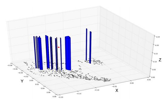
**Figure 7.** UAV environment. The starting positions are marked with a red point, and the destination positions are black shapes. The blue columns represent the no-fly zones, obstacles that must be avoided. The X, Y, and Z axes represent the longitude, latitude, and altitude coordinates measured in degrees for the lateral and kilometers for the vertical, respectively.
