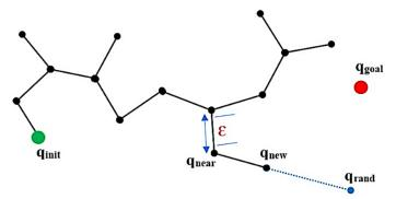
**Figure 2.** The construction process of RRT [25]. Input: Initial points  $q_{init}$ ,  $q_{goal}$ . Incremental distance  $\epsilon$ . Output: RRT graph G.
