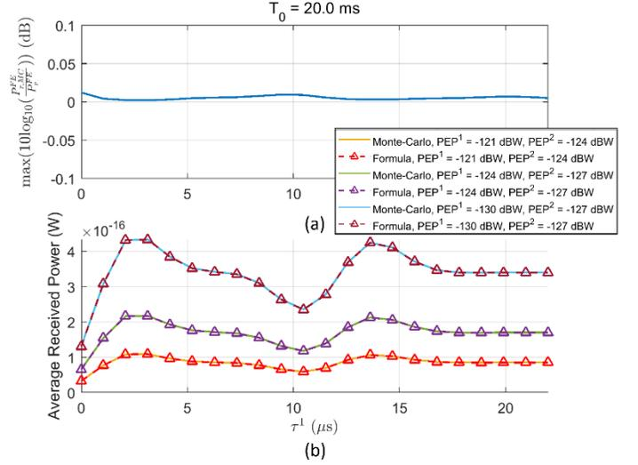
Fig. 9. (a) Results of the validation vector  $V^{fe}$  for the Monte-Carlo simulations under the fixed environment assumption and (b) outputs of  $P_{r,MC}^f(\tau^1)$  (in straight line) and  $P_r^f(\tau^1)$  (in dashed line) in W, for three different pairs (PEP<sup>0</sup>, PEP<sup>1</sup>).
