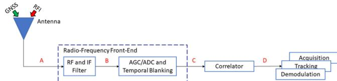
Fig. 1. Airborne GNSS DFMC generic receiver block scheme.
