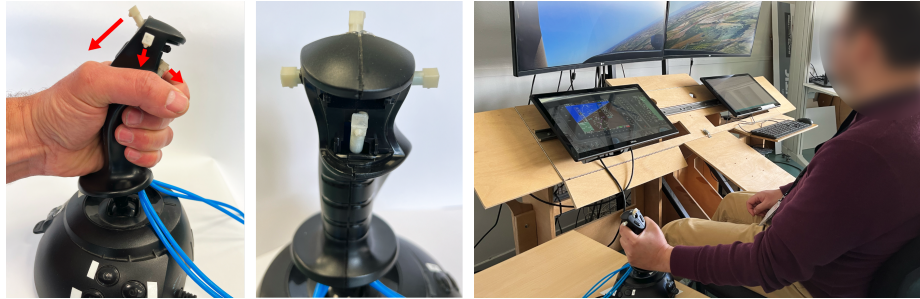
Fig. 1. On the left, the joystick gripped with the 4 nozzles (front, rear, left, right) on the upper part; center, the nozzles printed in white PLA are attached to the joystick by thermobonding and the pipes are integrated into the body of the device; right, the simulation platform.
