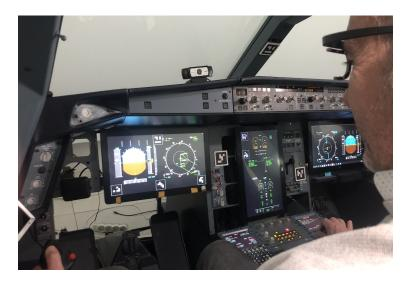
The ArUco marker pipeline has enabled real-time gaze mapping onto multiple screens and panels around pilot-in-command position while gaze analysis pipeline was identifying fixations and matching them with dynamic AOIs related to each instruments. To identify the relevant AOIs, a 3D model of the cockpit describing the AOI and the position of the markers has been realized (Figure 9).
