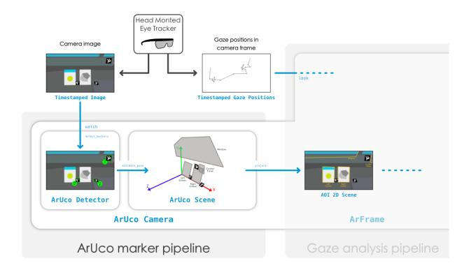
As illustrated in Figure 4, the first ArUcoCamera pipeline step is to detect all markers from a specific ARUCO dictionary<sup>2</sup> with a given size inside input image thanks to an ArUcoDetector instance.
