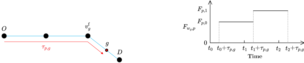
(a) Network representation of travel time from the origin O to a point g .
