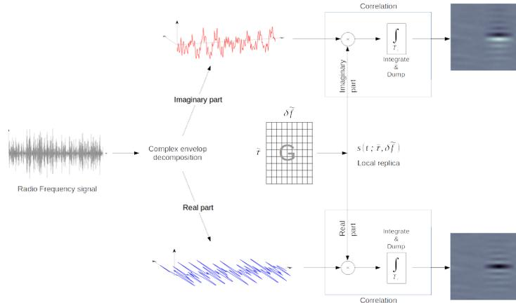
**Figure 2:** Correlator output images elaboration process. Firstly the received signal is divided into two orthogonal components. Then a grid  $G$  is generated from  $\tilde{\tau}$  and  $\delta\tilde{f}$  subset values.  $\tilde{\tau}$  and  $\delta\tilde{f}$  refer to the parameters of the local signal replica. The resulting 2D-images are used as an input for the CNN regression algorithm.
