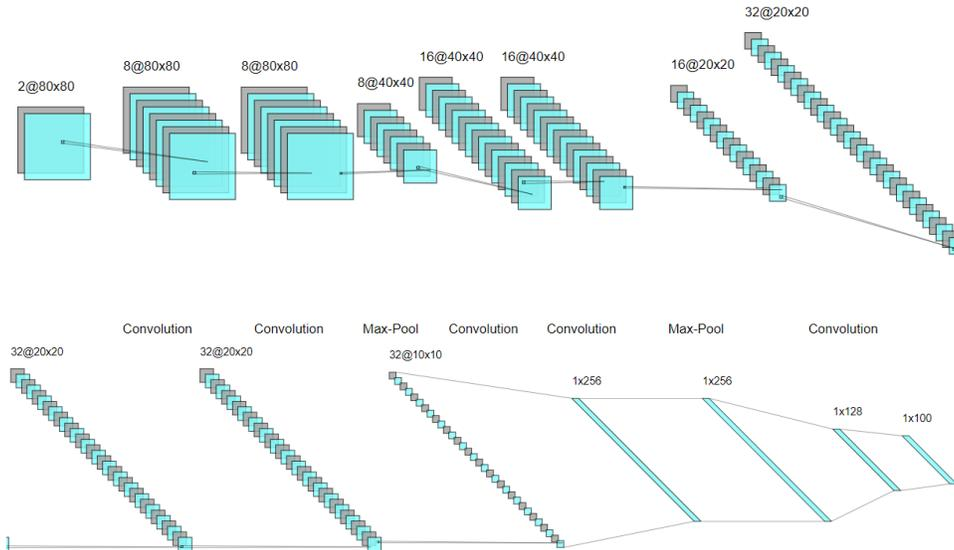
**Figure 3:** CNN architecture used for regression task with distributional outputs on 80x80 images. The top figure illustrates the first convolution blocks. Bottom figure shows the last convolution block followed by the dense layers with a multiple outputs layer. Images generated with NN-SVG LeNail (2019).
