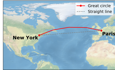
Fig. 2: Comparison between the straight line and the great circle trajectory between Paris and New York.
