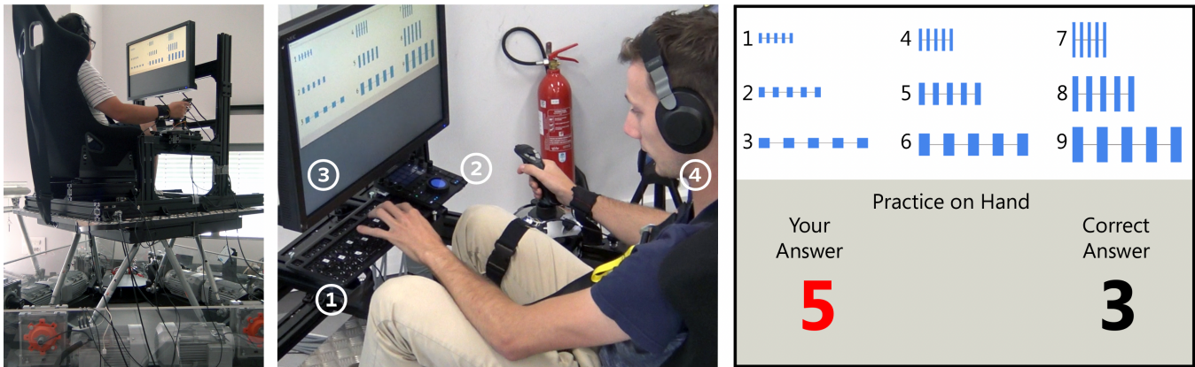
Figure 4: Experimental setup. Left: The 6 DOF motion platform ; Center: the experimental environment with a keyboard to indicate the number of the tacton (1), a Loupedeck CT pad for the design part (2), the screen (3) with the diagrams of the tactons and the anti-noise headphones (4) ; Right: the information screen during the training phase.
