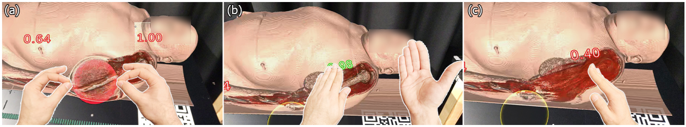
Figure 7: Prototype III: Refined colour tunnelling. (a) Persistent mode of colour tunnelling. (b) Tapping on the maximum value with one hand to enable adjustment and rotating the other hand to change the value. (c) Rotating the hand changes the entire tunnel's visibility range (compare the bone in b and c).
