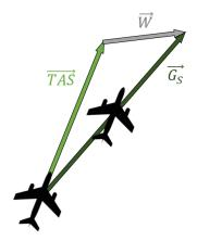
Fig. 20 The Wind Triangle graphically represents the relationships among velocity vectors used for air navigation. As the true airspeed  $\overrightarrow{TAS}$  gives the heading of the aircraft, the ground speed  $\overrightarrow{G_S}$  provides the trajectory of the aircraft (relatively to the ground).
