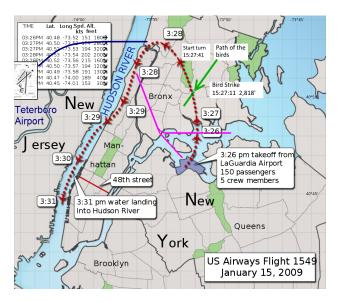
Fig. 1 US Airways Flight 1549. 2 minutes after take-off from LaGuardia airport, the aircraft struck a flock of Canada geese at an altitude of 2,818 feet. 5 minutes after take-off, the aircraft made an unpowered ditching into the Hudson River [2].
