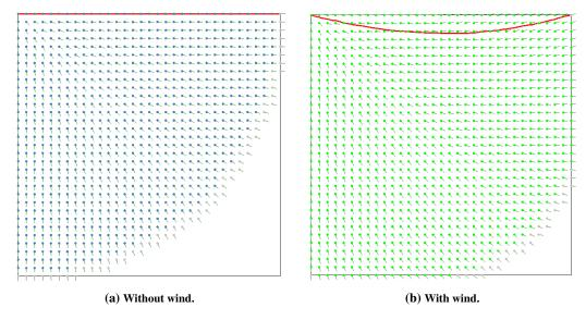
Fig. 23 Optimal trajectory generation in a wind field with the Fast Marching algorithm.
