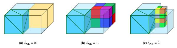
Fig. 12 Configuration of an octree node with a NorthEast neighbor with variable level difference  $\delta_{NE}$ .
