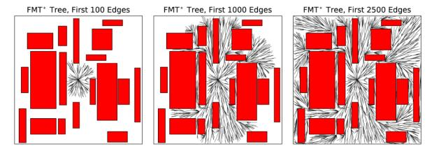
Fig. 25 The FMT\* algorithm [31, Fig. 1].
