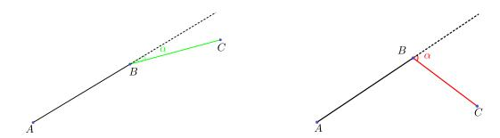
(a) The angle  $\alpha$  is small, the connection BC is possible.
