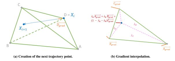
Fig. 19 Back propagation of gradients on a tetrahedron.
