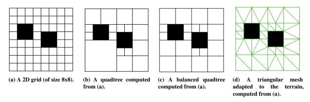
Fig. 5 Refinement of the data structure modeling a two-dimensional space.
