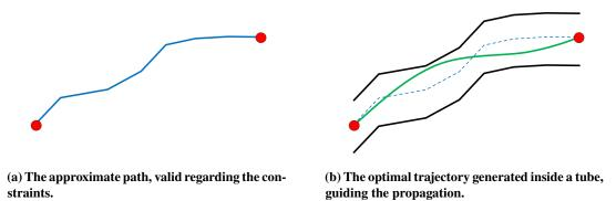
Fig. 24 Building of a guiding tube.
