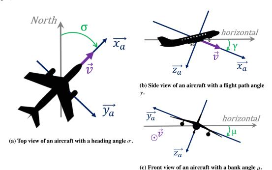
Fig. 4 The aerodynamic frame  $(\overrightarrow{x_a}, \overrightarrow{y_a}, \overrightarrow{z_a})$ . The frame origin is at the aircraft center of gravity, and the velocity vector  $\overrightarrow{v}$  (the aircraft true airspeed) is along  $\overrightarrow{x_a}$ .
