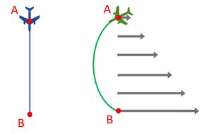
Fig. 22 Solutions to Zermelo's problem with constant wind (left) and with linearly variable wind (right).
