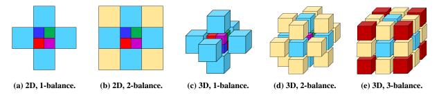
Fig. 10 Ways to balance a quadtree (a and b) or an octree (c, d and e). Adapted from [28, Fig. 5].
