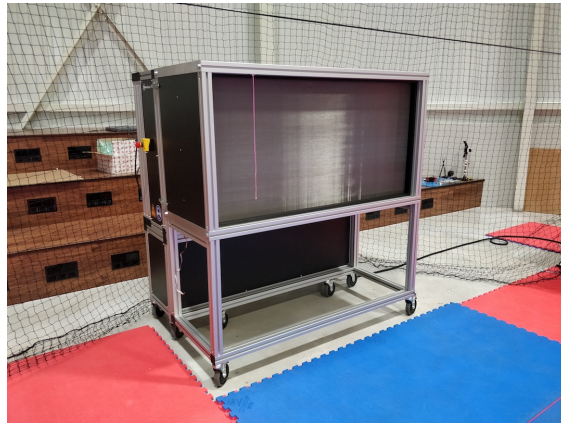
Fig. 3 WindShape, wind generator located inside ENAC's indoor flight facility.
