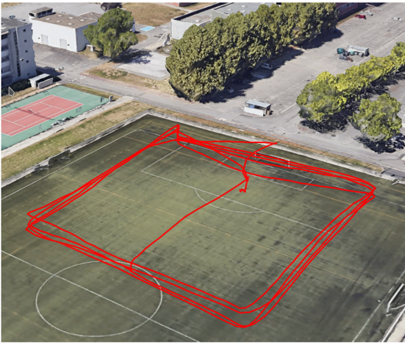
Figure 9. Square trajectory for the outdoor experiment. The four segments are 40 meters long. The flight speed is 2.5 or 5 m/s.
