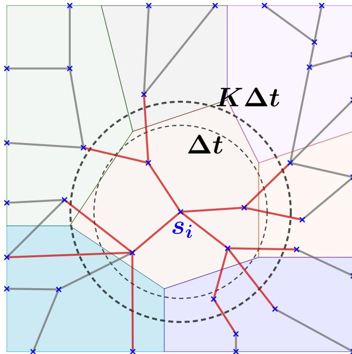
Figure 2: Capacity computation along time windows. We consider that a vehicle  $i$  consumes capacity of the sectors that are accessible from the start point  $s_i$  within a time less than  $K \Delta t$  (here: capacity is consumed only on red arcs).
