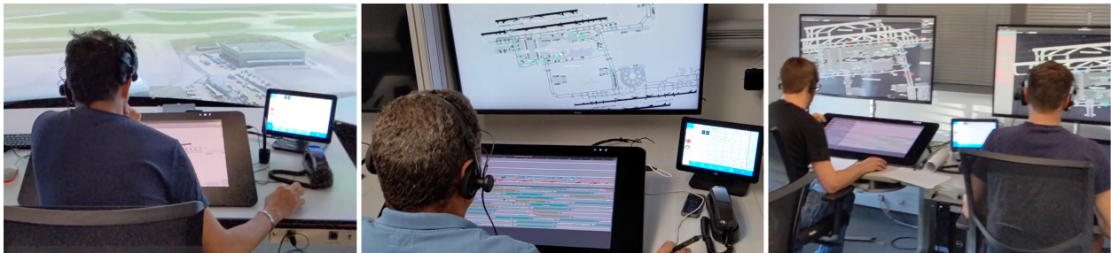
Figure 6: Experimental setup of the final assessment. Left: ATCO with the radar HMI and a realistic Paris-CDG tower simulation. Center: TFM with the supervision HMI and the radar HMI. Right: Pseudo pilots positions.
