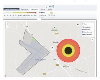
Fig. 2. The starting map: wind variator (1), which influences the buffers displayed on the map (2), other controls for safety analysis like trajectory definition, Geography and Drones tab (3), and the layers control with a small set of aeronautical data (4).
