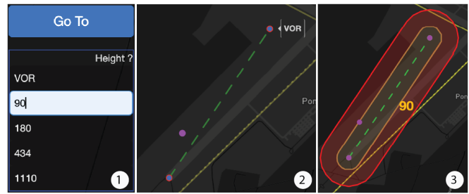
Fig. 4. The “GOTO” panel where buffers are automatically computed when height is changed (1), the nominal trajectory (2), and the resulting contingency and emergency buffers once displayed (3).
