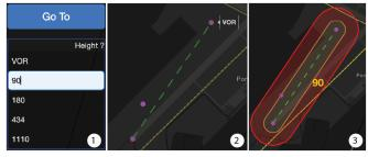
Fig. 4. The "GOTO" panel where buffers are automatically computed when height is changed (1), the nominal trajectory (2), and the resulting contingency and emergency buffers once displayed (3).
