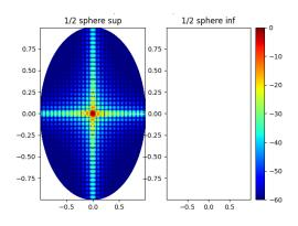
Fig. 5. Initial far-field of the uniform aperture on the sphere.
