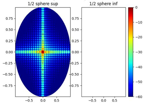
Fig. 5. Initial far-field of the uniform aperture on the sphere.
