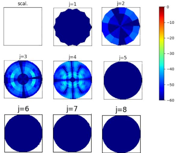
Fig. 8. Wavelet coefficients associated with the scaling function and the different wavelet levels for the horn antenna (dB).
