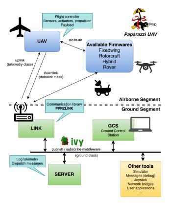
Figure 1 Paparazzi system architecture.
