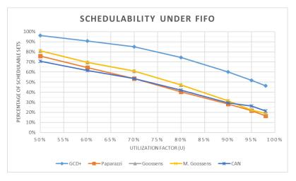
**Figure 10** Schedulability for 1000 filtered sets of 8 tasks, from U = 50% to 98%.
