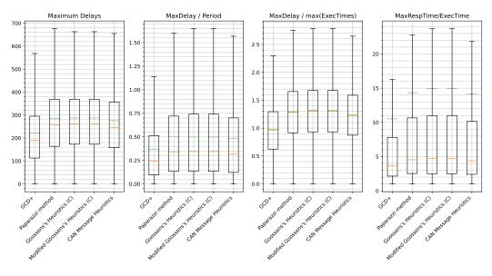
**Figure 7** Delays extracted from simulations for 1000 filtered sets of 8 tasks, with U = 95%.
