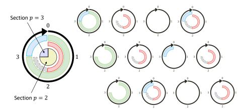
**Figure 5** Representation of the execution of  $\tau_1$  (green),  $\tau_2$  (blue),  $\tau_3$  (red) and  $\tau_4$  (dashed grey) over the overall GCD circle (left) and the cycles 0 to 11 composing the hyperperiod (right).
