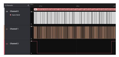
**Figure 13** Screen capture from the analysis of a Paparazzi telemetry case with a message loss at every 2 seeconds.
