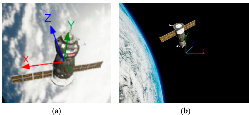
Figure 3. (a) Axis notation for a moving spacecraft frame, and (b) axis notation of the camera frame.
