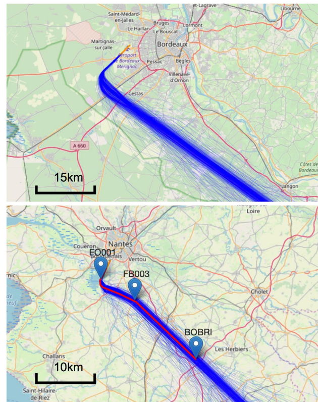
Fig. 10 This figure illustrates the departure procedure deformation. On top, the original trajectories at Bordeaux Airport are represented. At the bottom, the modified trajectories at Nantes Airport. In addition, the expected procedure following different aeronautical way points is shown in red
