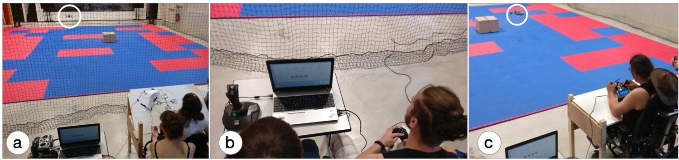
Figure 6: Workshop 1 performed in a flight arena with the first iteration of CandyFly (drones circled in white). a) P1 (cognitive and motor impairments) uses directional arrows with tactile zones via makey makey [17]; b) P3 (mild motor impairments) pilots with the video game controller; c) P4 (motor impairments) uses the radio control with extended 3D printed sticks.
