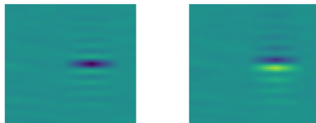
Figure 6: The I and Q correlator outputs of the synthetic data generator as images, PRN number set to 1
