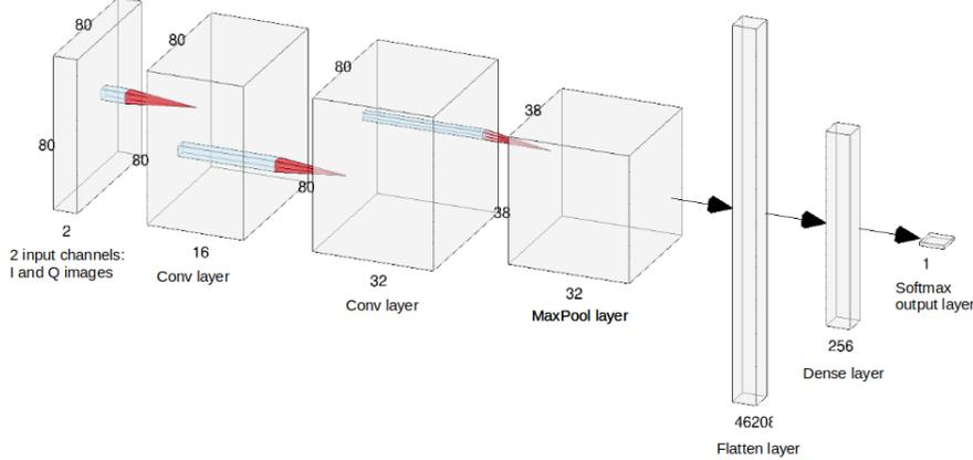
Figure 9: The CNN architecture used in this study: the input has 2 channels corresponding to  $I$  and  $Q$  channels, the first and second convolutional layers have 16 and 32 filters respectively with ReLu activations and the pooling layer is a  $2 \times 2$  max pooling operation layer (this figure has been generated by the NN-SVG tool (LeNail, 2019)).
