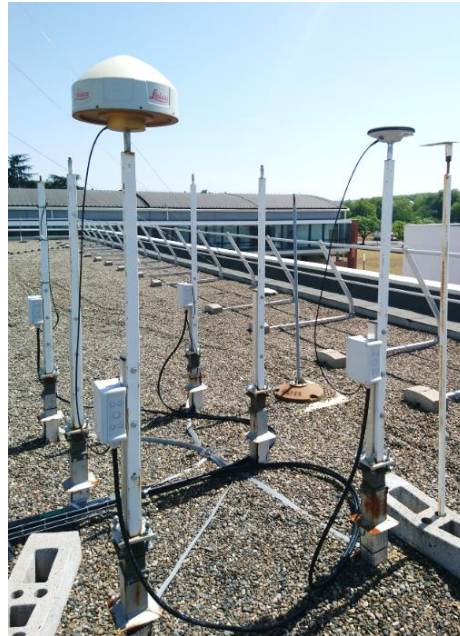
Figure 4 – Photos of the choke-ring antenna on the roof of an ENAC building
