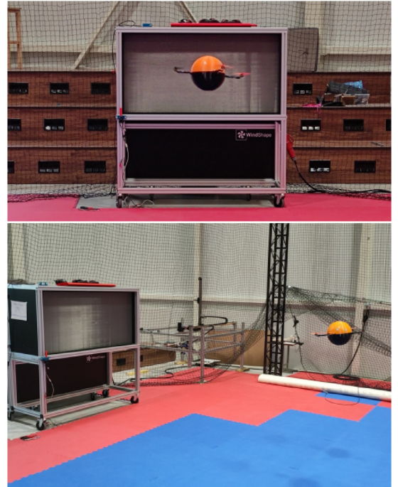
Figure 3. Quadrotor during calibration in front of the WindShape wind generator
