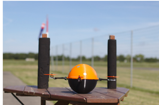
Figure 2. Quadrotor with custom spherical body shape.
