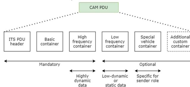
Figure 1 – CAM payload
