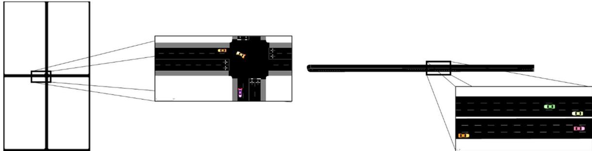
**Figure 5 – Two SUMO layouts: urban (left), and 3km highway (right)**
