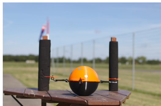
Figure 2: Quadrotor with custom spherical body shape
