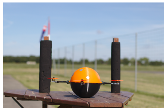
Figure 2: Quadrotor with custom spherical body shape
