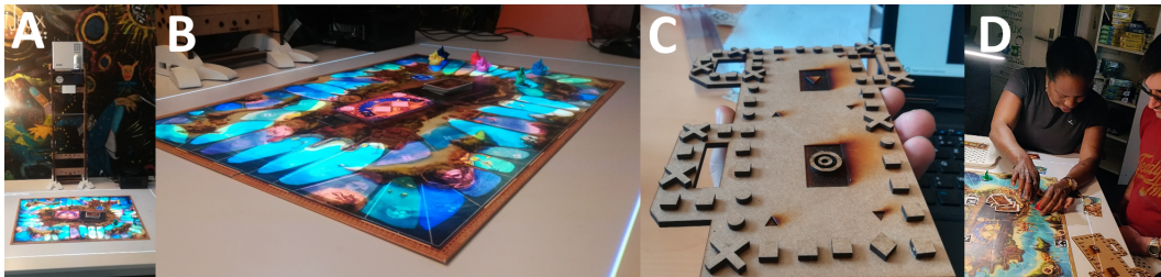
Fig. 1. JamaicaAR is an inclusive version of the Jamaica board game using both handcrafted fixes done by professionals of board game adaptations, as well as interactive augmentation through SAR. A) PapArt hardware [31] and Jamaica board, B) projection of areas detecting pawns with a color-depth camera. Areas are touch sensitive and trigger audio feedback, C) a tactile memory aid of the spatial layout of the board, D) people with visual impairments playing JamaicaAR.
