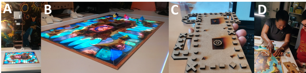
Fig. 1. JamaicaAR is an inclusive version of the Jamaica board game using both handcrafted fixes done by professionals of board game adaptations, as well as interactive augmentation through SAR. A) PapArt hardware [31] and Jamaica board, B) projection of areas detecting pawns with a color-depth camera. Areas are touch sensitive and trigger audio feedback, C) a tactile memory aid of the spatial layout of the board, D) people with visual impairments playing JamaicaAR.
