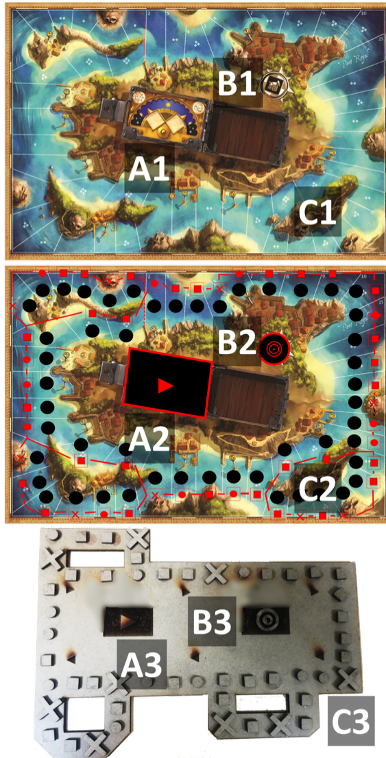
Fig. 4. Board adaptation and memo. Top: The original Jamaica board. Middle: JamaicaAR Board with the transparent relief (in red on the picture for better visibility), and the "wavy" transparent tactile pattern for the interactive zones (in black on the picture). The visual dice areas (A1 and B1) are transcribed as the interactive area for launching the dice of the morning and night action (A2) and the fight dice (B2). Bottom: the memo (A5 size) presents an overview of the paths on the board. The relative position of the dice areas are represented with the same relief symbols (A2/A3 with a "play" triangle and B2/B3 with the target). Triangles are engraved every 5 spaces to facilitate counting the number of the spaces. The alternative paths are represented (C1, C2 and C3) for a better layout overview.
