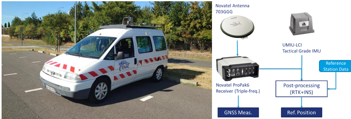
Figure 7 Test car for data collection (left) and equipped sensor (right)
