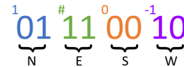
Figure 12: Level differences are coded with 1 byte (8 bits), with 4 duets of bits each corresponding to a cardinal direction in space.
