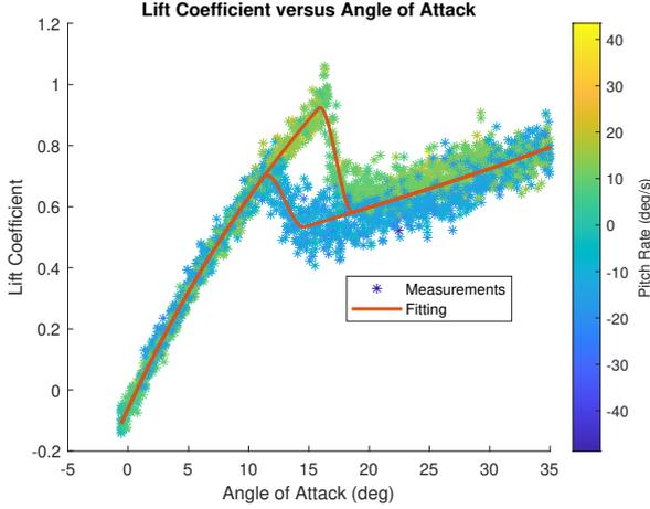
Fig. 3. The fitting results on the experimental data
