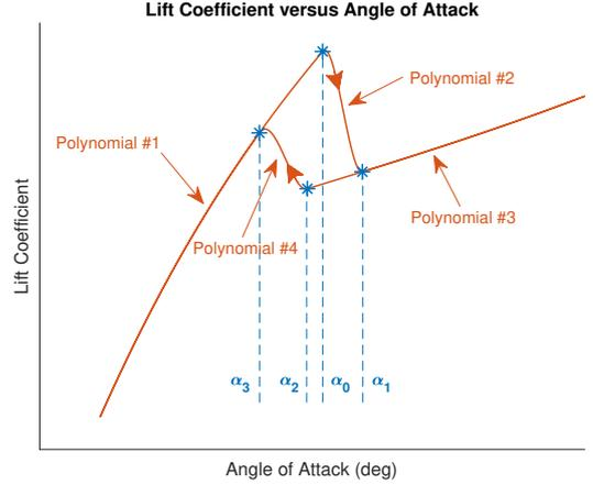
Fig. 1. The proposed model for the lift coefficient
