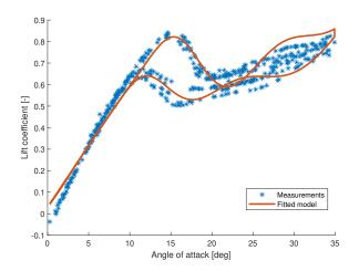
Fig. 2. Global model fitting using the SVR non-parametric method on the validation dataset
