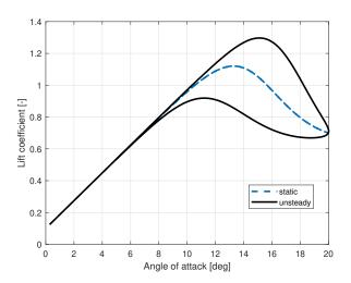
Fig. 1. Typical dynamic stall behaviour, based on (8)
