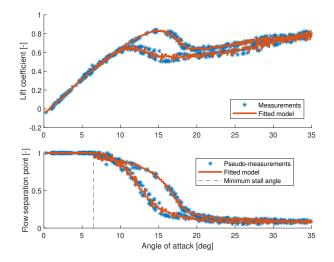
Fig. 4. Separated method fitting using the RT non-parametric method on the validation dataset
