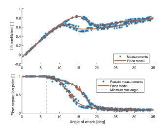
Fig. 3. Separated method fitting using the GP nonparametric method on the validation dataset
