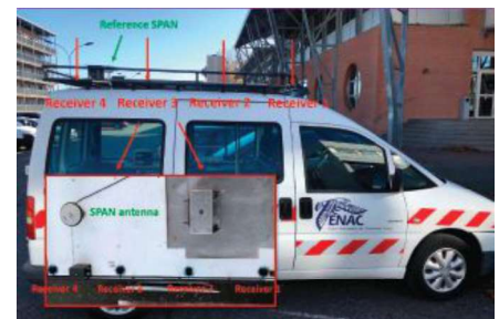
FIGURE 2 Real data collection set-up: Four GNSS U-blox antennas and one NovAtel SPAN receiver antenna on the vehicle rooftop.
