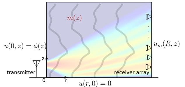
Fig. 1. Schematic of the bistatic configuration. Initial field  $\phi(z)$  propagates rightward in horizontally stratified atmosphere, which is characterized with refractivity  $m(z)$ . Our goal is to retrieve  $m(z)$  from wavefield measurements obtained with receiver array at distance  $R$  from the known source.
