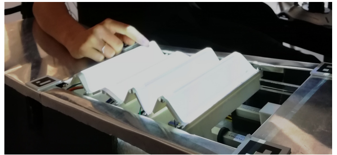
Figure 6: The flexible surface during the surveillance task. On the picture, the user is tapping the last fold to modify the corresponding parameter's state.
