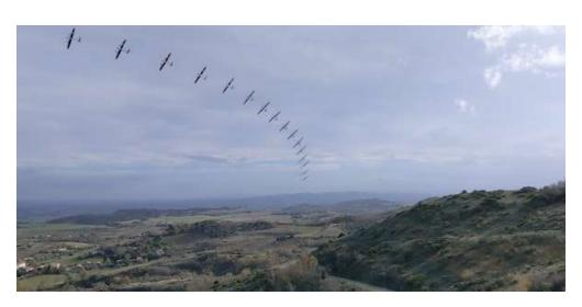
Fig. 7 Sequential imaging of the glider during the inclined circle trajectory, climbing upwind towards positive wind gradient.
