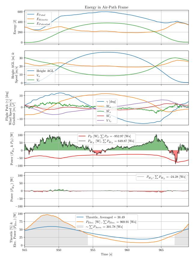
Fig. 12 Energy cycle and wind gradient power during a full cycle with emphasis on the contribution of horizontal wind gradient  $\dot{w}_x$  during ascend towards positive wind gradient and descend towards negative wind gradient.
