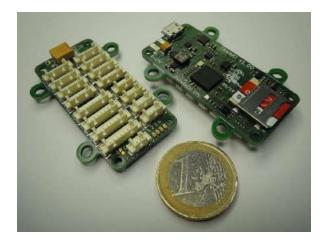
Fig. 3 3D view of the final design of the Tawaki autopilot
