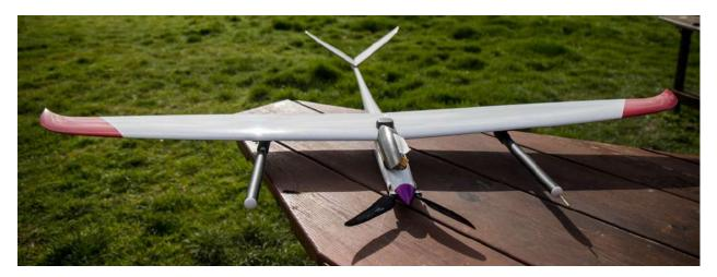
Fig. 2 A close-up view of the vehicle with Smart-Probe 5-hole probe is shown in the picture.
