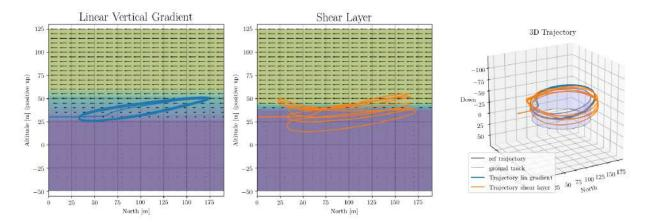
Fig. 14 Simulation of inclined circle trajectory inside linear vertical wind gradient on the left, thin wind shear layer in the middle, and the 3D trajectories of the two cases with respect to desired reference trajectory is shown.
