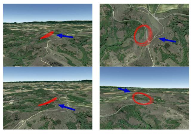
Fig. 9 Real flight trajectory of the inclined circle, controlled by *Paparazzi Autopilot*, direction of the wind is shown.
