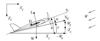
Fig. 8 Air-path relative velocity and longitudinal forces on a vehicle in uniform wind.
