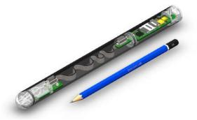
(b) Smart-Probe design with internal electronics.
