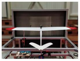
(b) Dynamic calibration and wing up-wash effect correction in front of ENAC WindShape.
