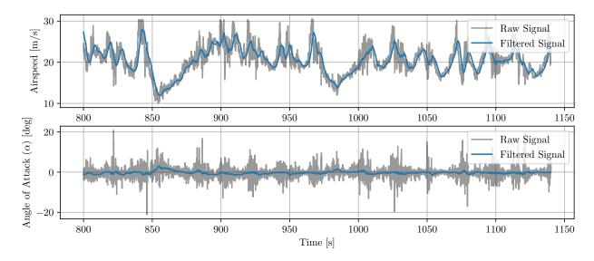
Fig. 11 Nature of measured airspeed and angle of attack signal from flights, compared to filtered signal.
