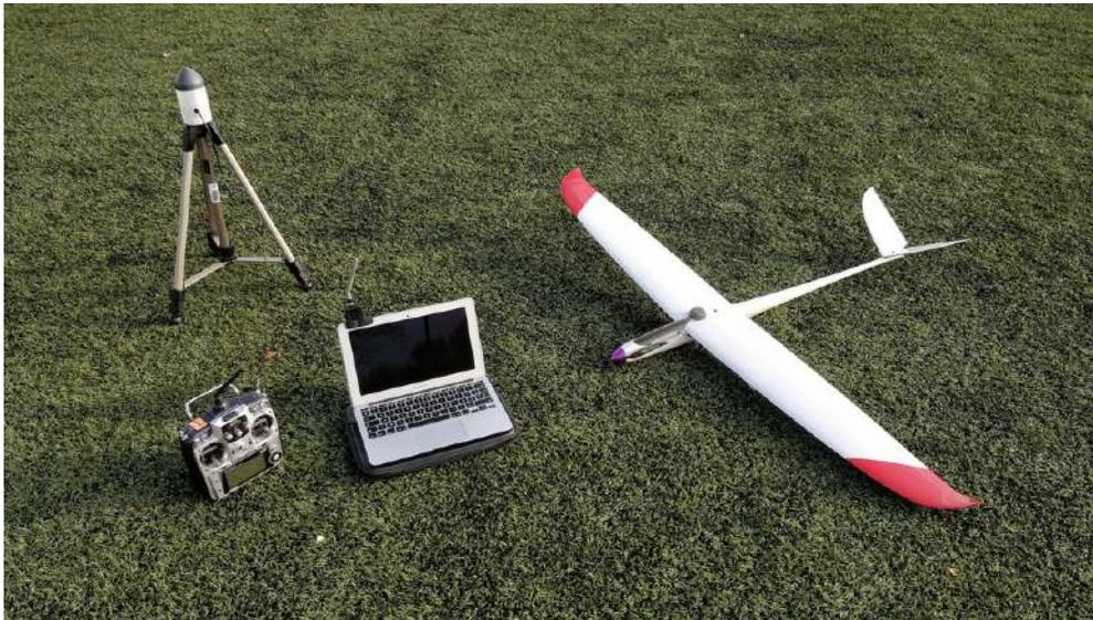
**Fig. 1** System overview of the components used during the flight tests.
