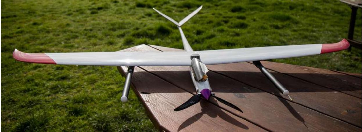
Fig. 2 A close-up view of the vehicle with *Smart-Probe 5-hole probe* is shown in the picture.
