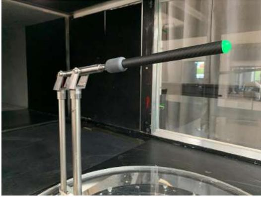
(a) Static calibration inside ISAE SABRE low-Re wind-tunnel.
