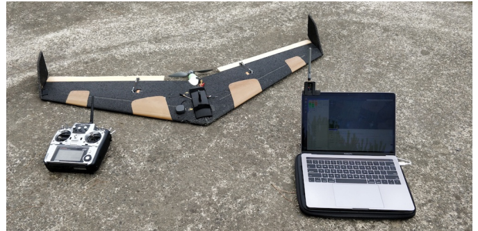
Fig. 1. Complete flight test system that is used during the data set collection and real-time detection flights. Note the small Xbee radio modem attached on the side of the computer screen, used for telemetry communication between the aircraft and the Ground Control Station
