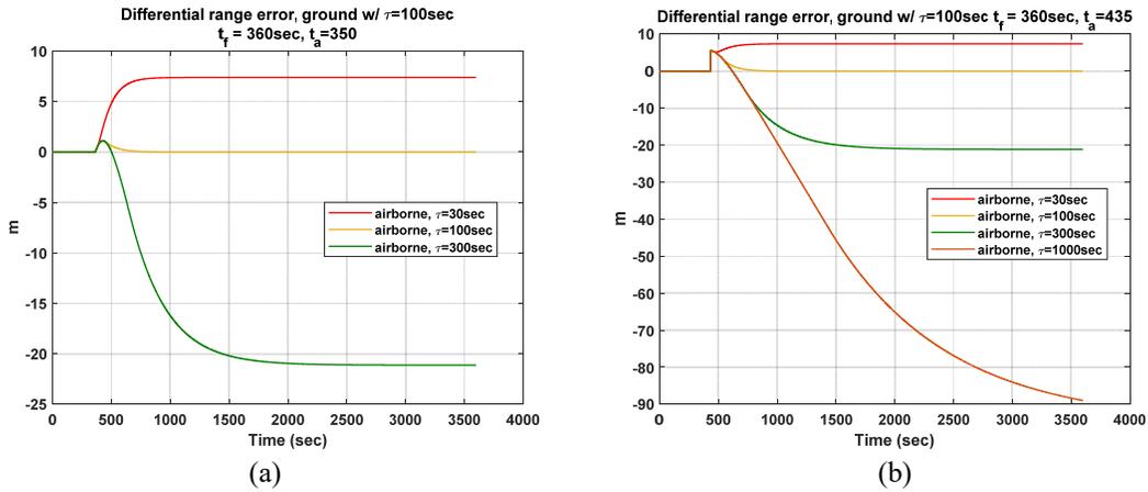
Figure 2 Time history of the differential range error due to the CCD faults when a fixed time constant is used at the ground (100 seconds) for various time constants at the airborne, (a)  $t_a < t_f$ , and (b)  $t_a \geq t_f$  cases
