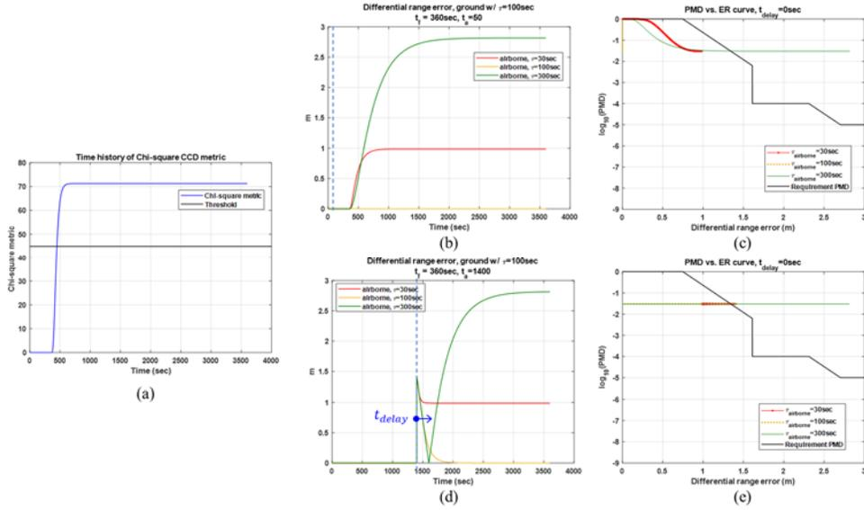
Figure 6 (a) Time history of the CCD monitor and its threshold, (b, c) Time history of the differential range error and the PMD vs. ER requirement curve for  $t_a < t_f$ , and (d, e) Time history of the differential range error and the PMD vs. ER requirement curve for  $t_a \geq t_f$ . The vertical dashed blue line indicates the  $t_{\text{delay}}$ , and  $d_{\psi}$  and  $d_{\phi}$  are set to  $-0.01$  m/s and  $-0.002$  m/s, respectively.
