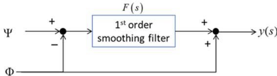
Figure 1 Block diagram of carrier smoothing filter
