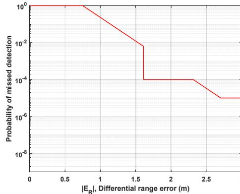
Figure 4 PMD constraints according to differential range error
