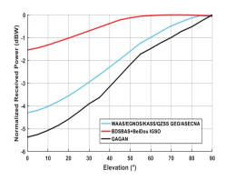
The figure above shows the normalized Received Power vs Elevation (MEO upper, GEO lower).
