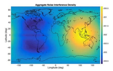
The worst case is located at (7.5°N,117.5°E) in South East Asia with a value of -200.38 dBW/Hz for a BPSK10 and BW2=12 MHz Receiver
