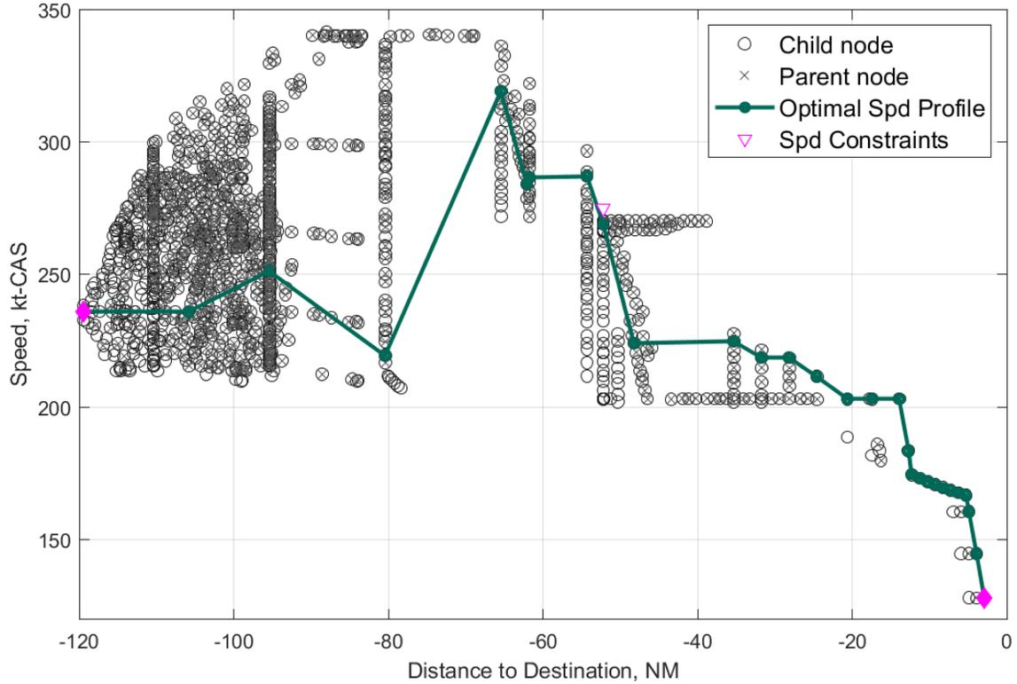
**Fig. 4 Search Space after calculation. The optimal speed profile (green-dotted line), children and parent nodes, speed constraints (magenta triangles) and the initial and target nodes (magenta diamonds).**
