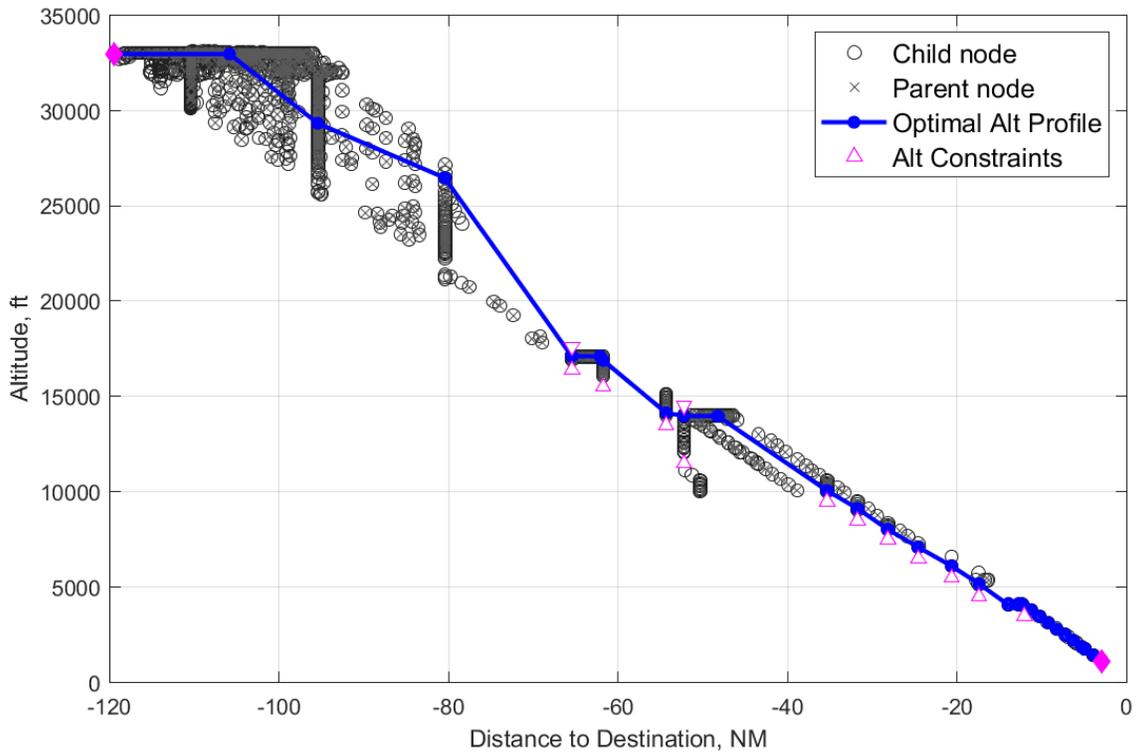
**Fig. 3 Search Space after calculation. The optimal altitude profile (blue-dotted line), children and parent nodes, altitude constraints (magenta triangles) and the initial and target nodes (magenta diamonds).**
