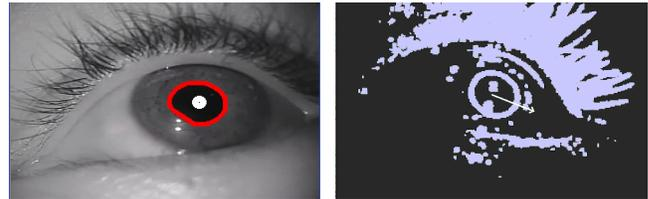
**Figure 1: (Left) Pupil center detected from an IR head-worn eye tracker. (B) Using an unmodified camera, the eye movements are estimated based on the overall movement of the eye using the Lucas-Kanade optical flow algorithm.**
